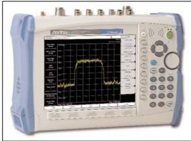
provides a 20 MHz demodulation capability to measure technologies such as LTE and WiMAX, and a 30-MHz Zero-Span IF Output for external demodulation of virtually any other wideband signal. In addition, a Vector Signal Generator option with the flexibility to generate two modulated signals plus noise is available for comprehensive receiver testing.
