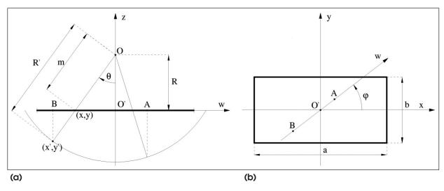
Figure 3 • Cross-sections of a flat, rectangular reflector with feed placed at O.
