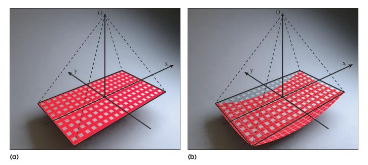
Figure 2. Integration areas for integral A (a) and B (b) marked with red color.
