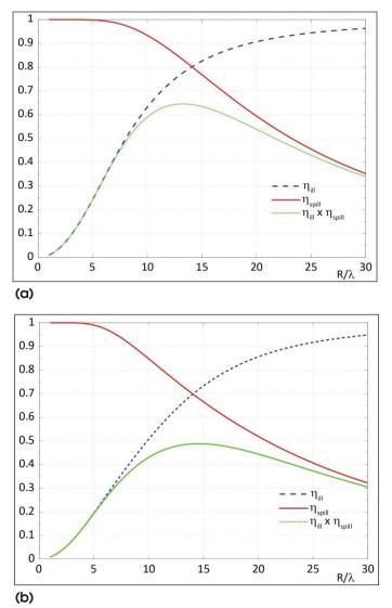
Figure 6 • Spillover efficiency (solid red line), illumination efficiency (dashed blue line) and their product (dotted green line) for the rectangular reflective array, Example 2 (a). Corresponding efficiencies for a reflectivearray with feed pattern parameters:  $q_{\rm e} = 5$ ,  $q_{\rm H} = 10$  (b).
