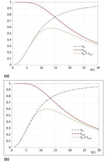
Figure 5 • Spillover efficiency (solid red line), illumination efficiency (dashed blue line) and their product (dotted green line) for the rectangular reflectivearray, Example 2 (a). Corresponding efficiencies for a circular reflectarray (b).
