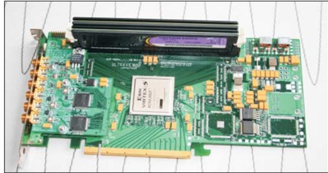
remotely, modify the board's standard data acquisition VHDL firmware to perform advanced application specific hardware signal processing, including filtering, sub-band tuning, averaging, spectroscopy, SDR and image processing. This modular VHDL source is available to OEM users under NDA.
