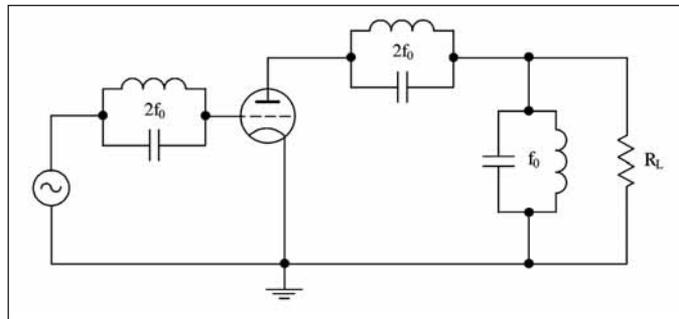
Figure 5 · Biharmonic power amplifier with input second-harmonic resonator.
