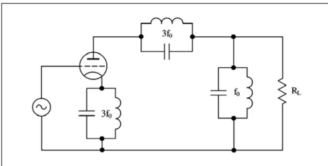
Figure 9 · Bi-harmonic power amplifier with cathode harmonic control.
