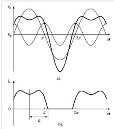
**Figure 6 . Input and output voltage and current waveforms with second harmonic.**
