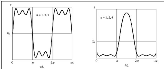
Figure 2 · Fourier voltage and current waveforms with three harmonics.
