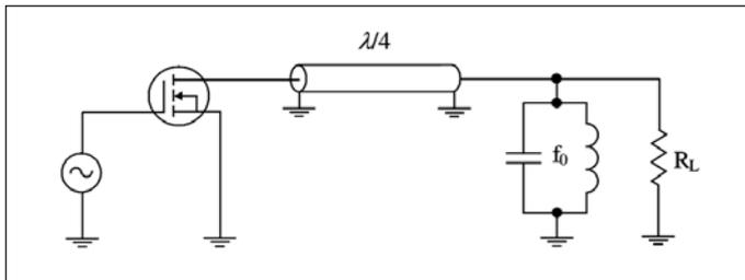
Figure 11 - Class F power amplifier with series quarter-wave transmission line.
