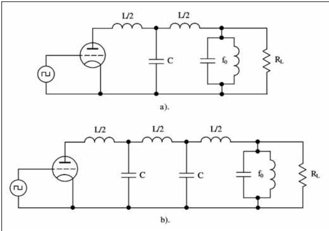
Figure 7 · Bi-harmonic and polyharmonic vacuum-tube power amplifiers with low-pass filters.
