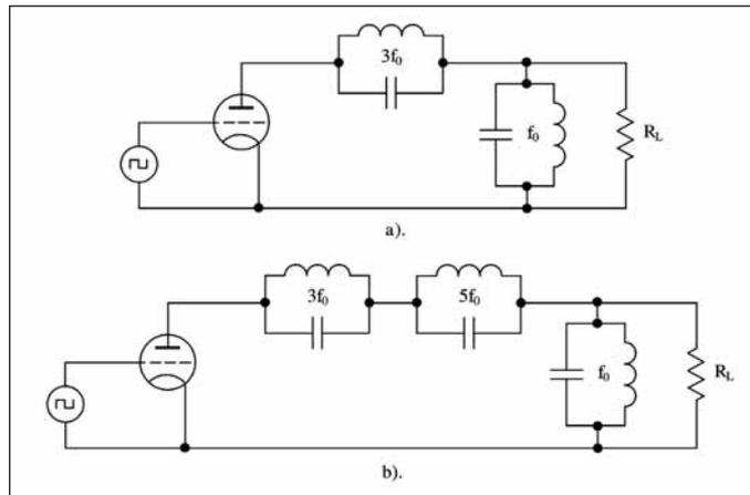
Figure 3 · Biharmonic and polyharmonic vacuum-tube power amplifiers with odd-harmonic resonant tanks.
