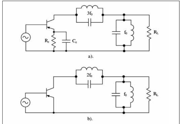
Figure 8 · Bi-harmonic bipolar-transistor power amplifiers.
