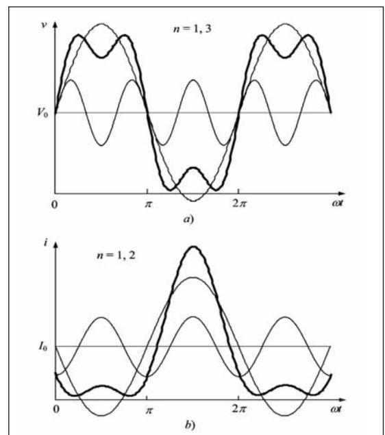
Figure 1 · Fourier voltage and current waveforms with third and second harmonics.
