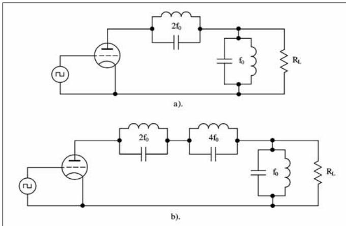
Figure 4 · Biharmonic and polyharmonic vacuum-tube power amplifiers with even-harmonic resonant tanks.
