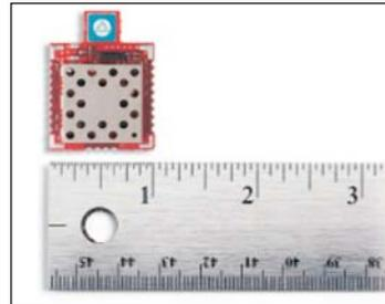
power consumption transceiver module. Power output is variable from 0 to 100 mW, with maximum current draw
