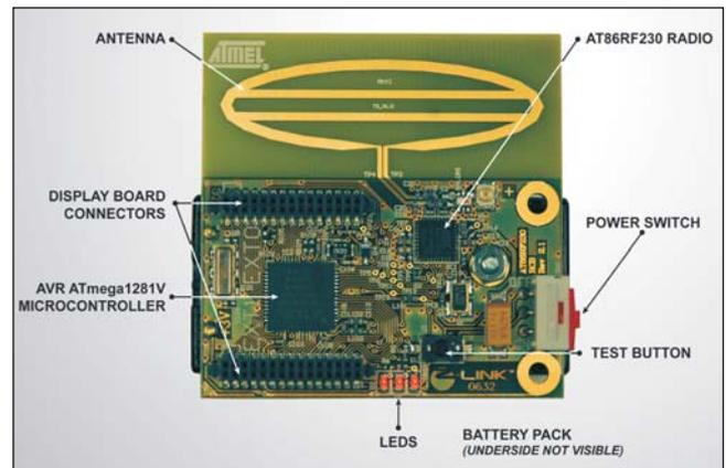
ment with a ZigBee/IEEE 802.15.4 system. The major components—transceiver IC, low power MPU, antenna and interconnections are evident in the photo.
