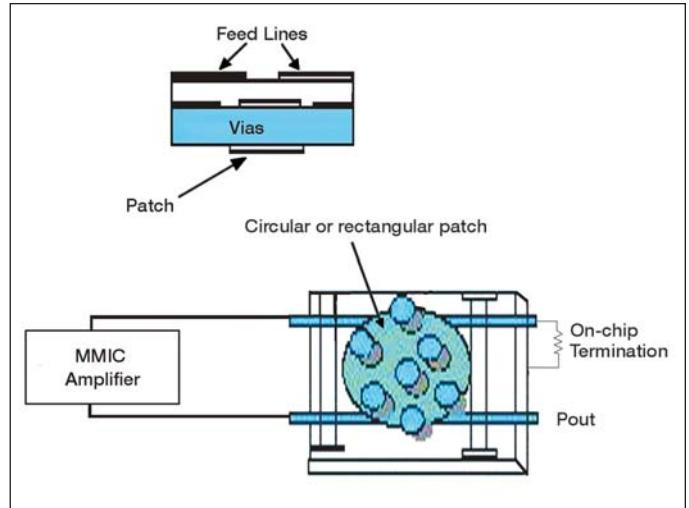
**Figure 7 . Combination of the active antenna and oscillator.**
