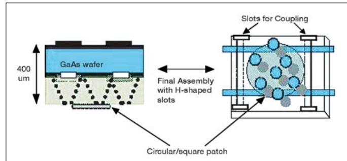
**Figure 6 . Active antenna design using slot coupling to the GaAs wafer.**
