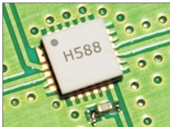
Figure 1 - Photograph of the HMC588LC4B Wideband VCO in a 4 x 4 mm SMT package, mounted to a PC board.
