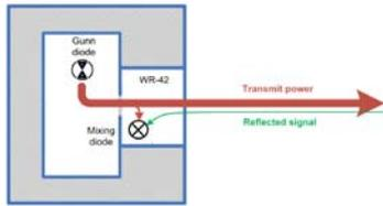
Fig. 3. Sensor front-end module illustration.
