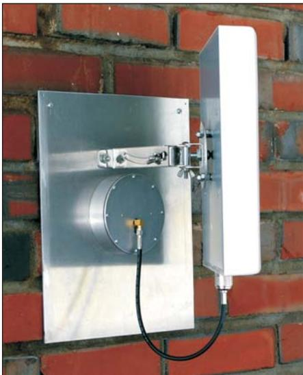
Figure 2 · A wall coupler with WLAN antenna, installed on a brick wall.
