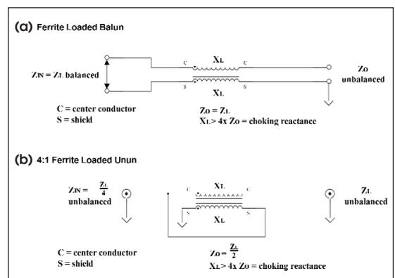
Figure 2 · (a) Ferrite-loaded transmission line used as a balun, and (b) a ferrite-loaded 4:1 transmission line transformer.
