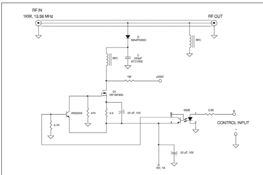
Figure 6 · A high power PIN diode switch circuit.
