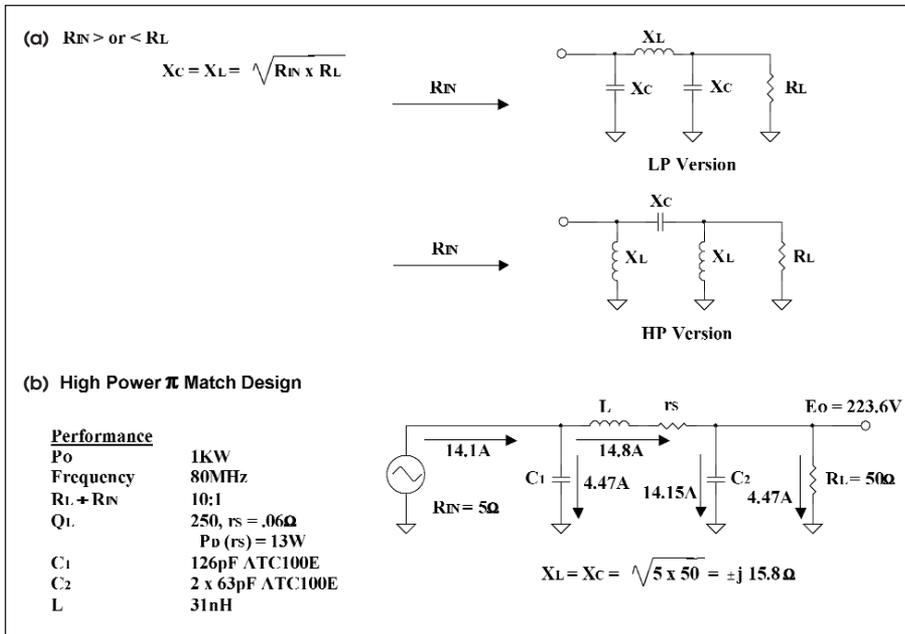
Figure 5 · High power pi network matching circuits. (a) shows the high-pass and low pass configurations; (b) is a high power pi network for a 10:1 transformation and 90-degree phase shift.
