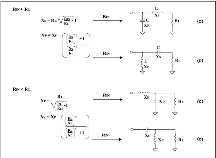
Figure 4 · LC Matching networks: (a) and (b) provide transformation to a load resistance lower than  $R_{in}$ , while (c) and (d) provide transformation to higher resistances.
