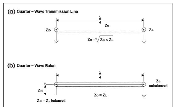
Figure 1 · (a) A quarter-wave transmission line transformer, and (b) a quarter-wave line used as a balun.
