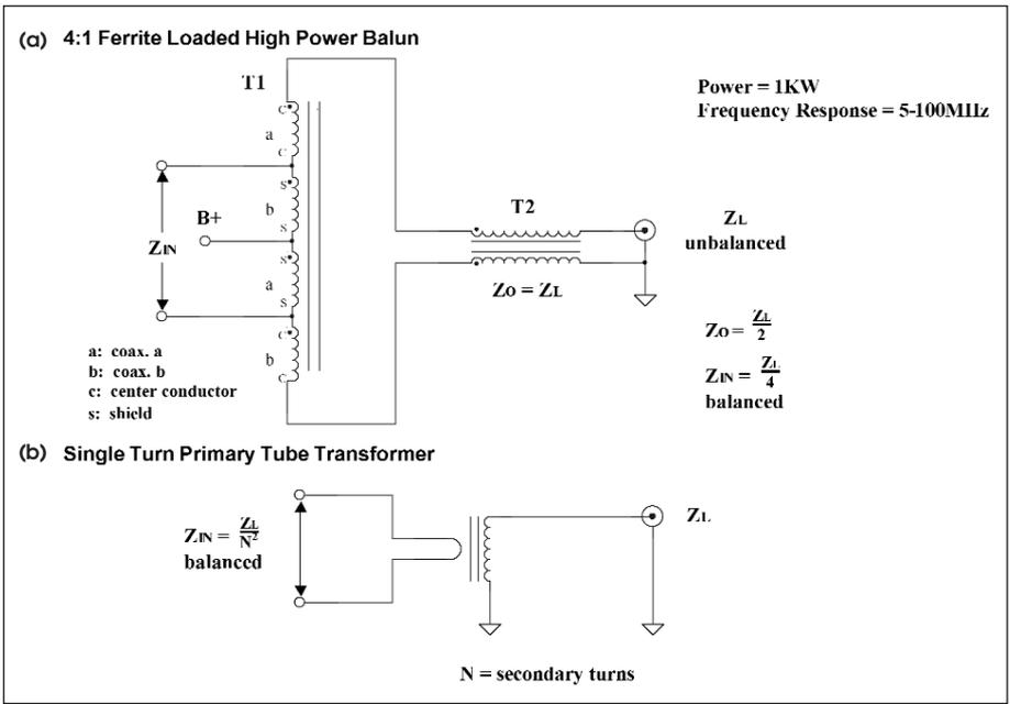
Figure 3 · (a) An improved high power 4:1 transformer with a separate balun, and (b) a conventional transformer with tightly-coupled windings.
