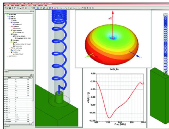
Complex geometries such as this fully-parameterized, variable-pitch helix antenna can be designed quickly with HFSS v9.
