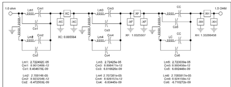
Figure 10 · The network after equalizing the inductor values.
