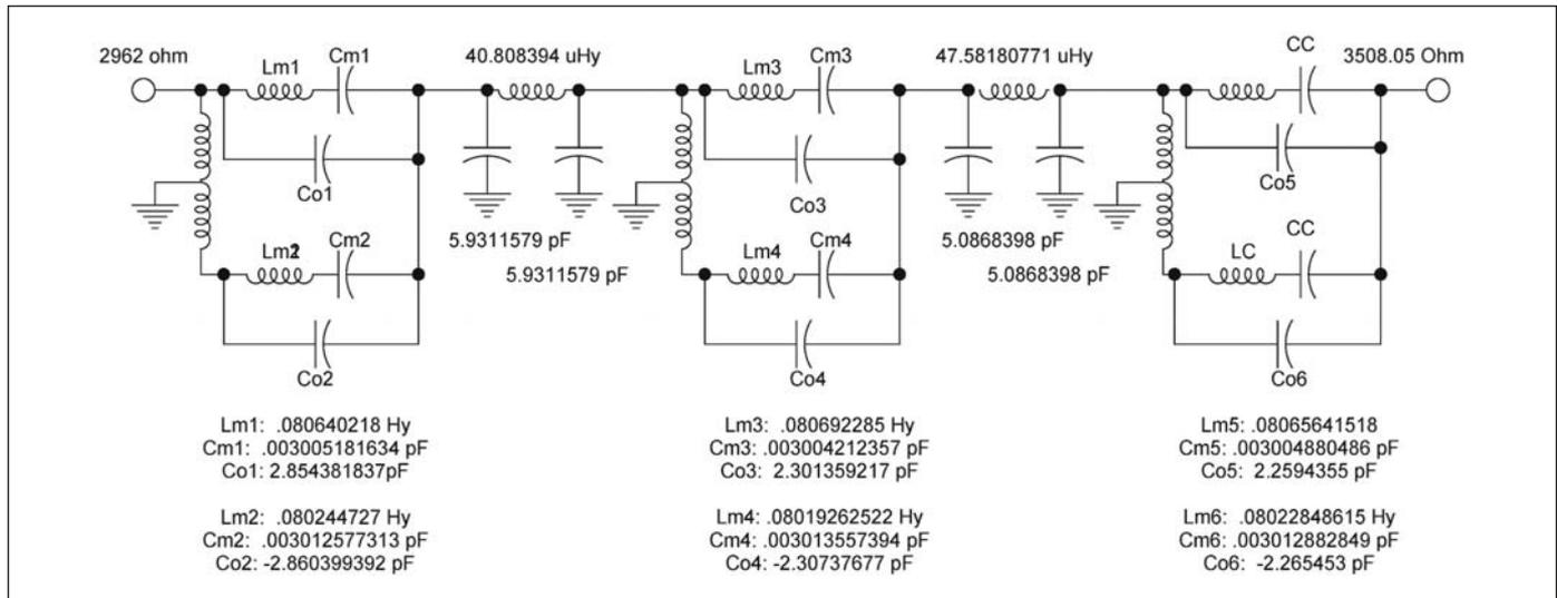
Figure 11 . The final bandstop filter network, after scaling for the desired motional inductance and making impedance inverter substitutions.
