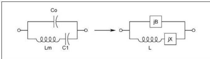
Figure 2 · Approximate bandpass to lowpass transformation of a crystal resonator.
