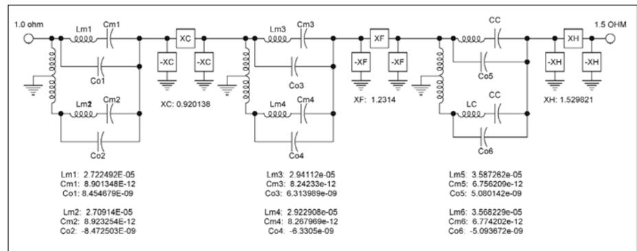
Figure 9 · Bandstop network after simplification.
