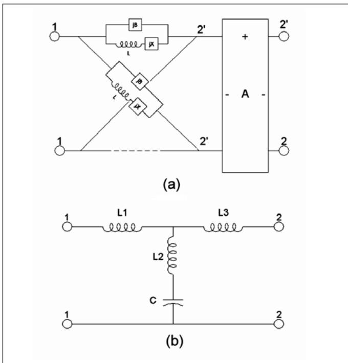
Figure 3 · (a) Second order low-pass section of inductances and frequency independent susceptances. (b) An LC ladder equivalent to (a).
