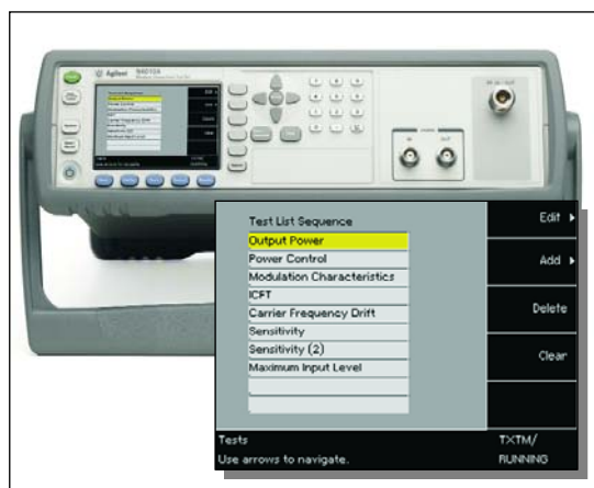
With Option 101, the Agilent N4010A handles Bluetooth production testing.
