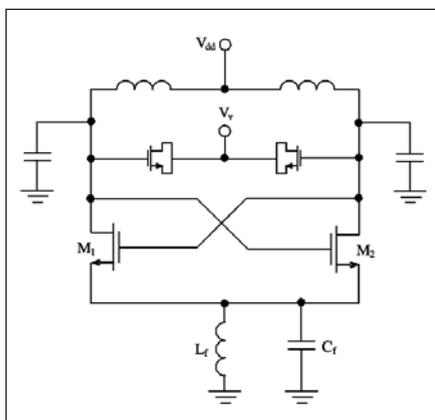
Figure 23 · Differential voltage-biased VCO with noise filter.
