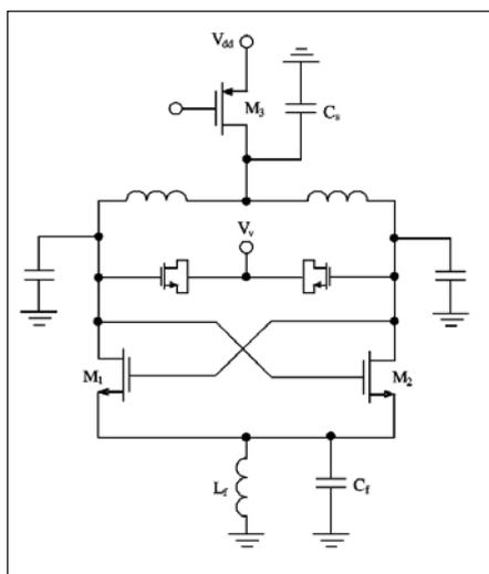
Figure 22 · Differential top-biased VCO with complete noise filter.
