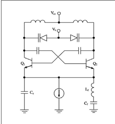
**Figure 25 · Differential tail-biased VCO with second harmonic trap.**
