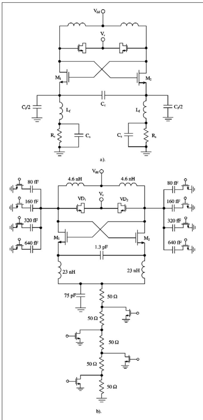
Figure 24 . Differential VCO with noiseless current sources (23).
