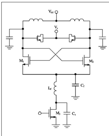
Figure 21 · Differential tail-biased VCO with complete noise filter.
