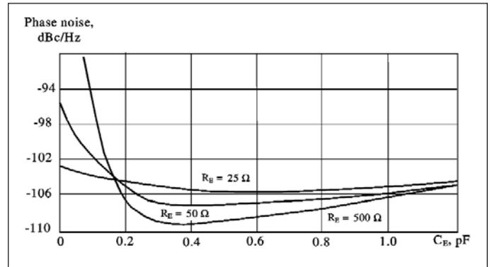
Figure 15 · Simulated phase noise of LC oscillator with emitter degeneration.
