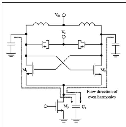
Figure 20 · Differential tail-biased VCO with capacitive noise filter.
