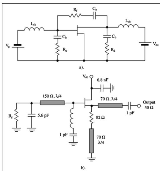
Figure 13 · Diagram of a low frequency circuit reducing phase noise.
