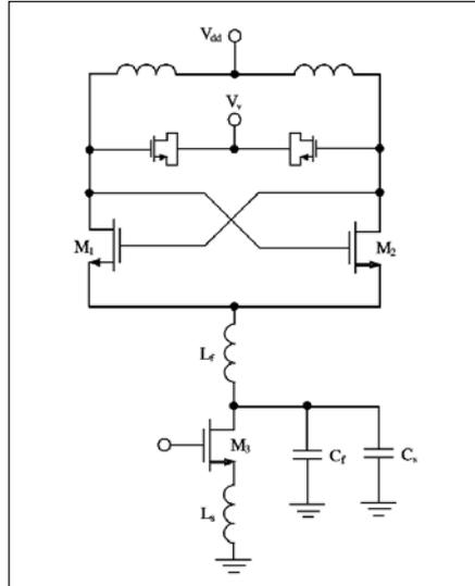
**Figure 26 · Differential VCO with tail current noise suppression.**
