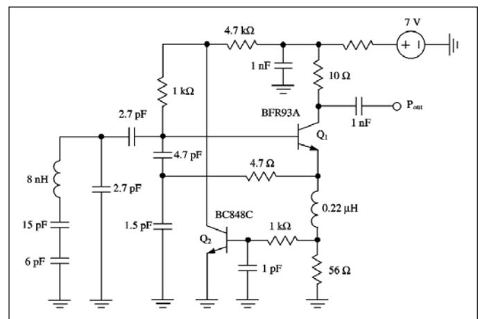
Figure 16 · Bipolar oscillator schematic with emitter noise feedback (18).
