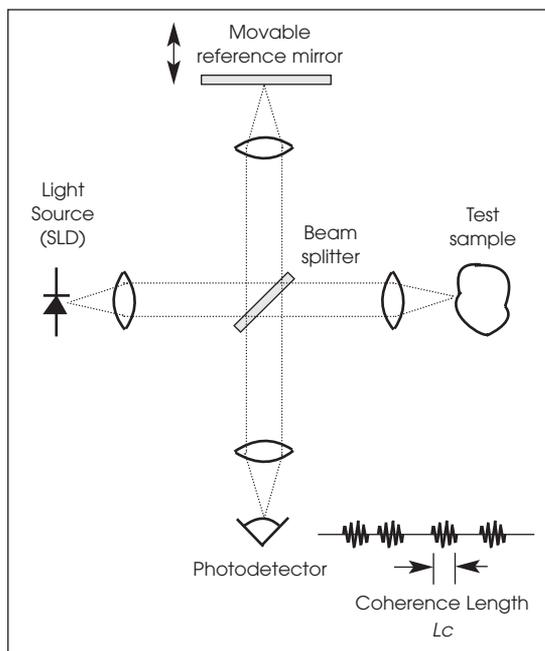
Figure 1 · Typical features of an OCT system.
