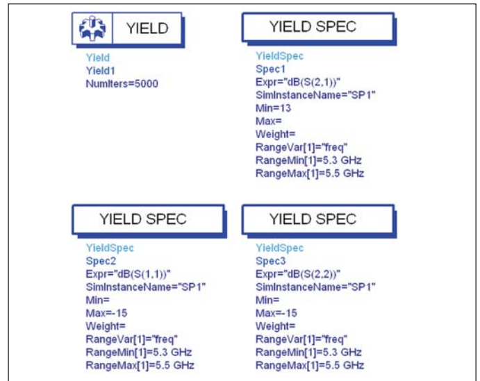
Figure 2 · Yield analysis setup for statistical analysis in simulation.
