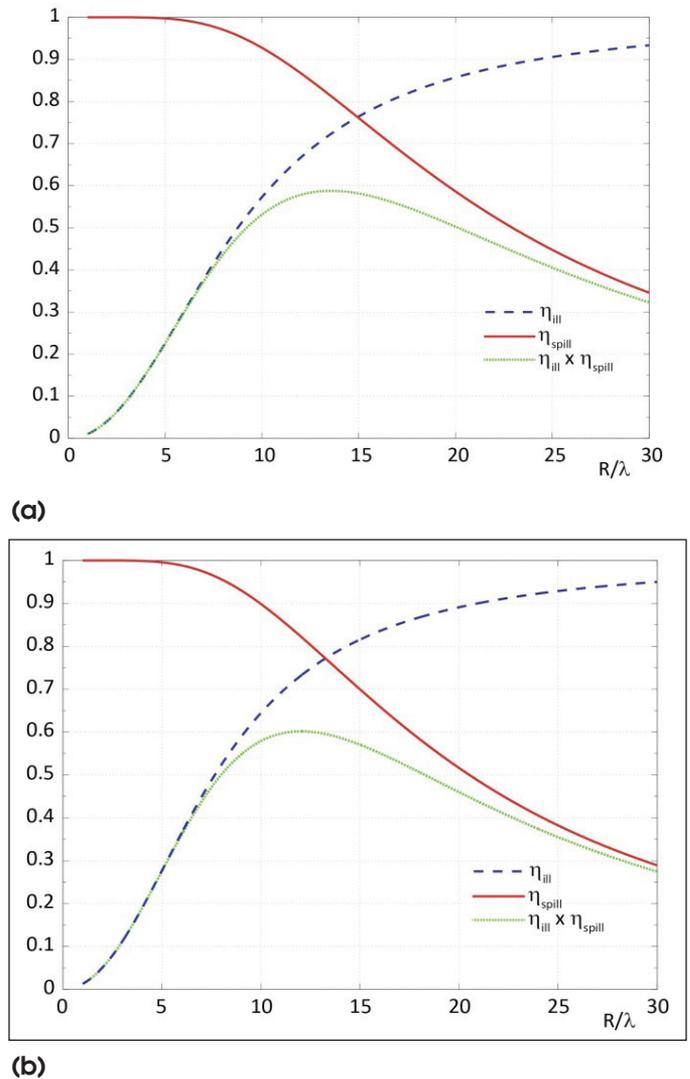
**Figure 5 • Spillover efficiency (solid red line), illumination efficiency (dashed blue line) and their product (dotted green line) for the rectangular reflectivearray, Example 2 (a). Corresponding efficiencies for a circular reflectarray (b).**
