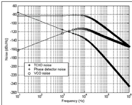
Figure 3 · TCXO, phase detector and VCO noise.
