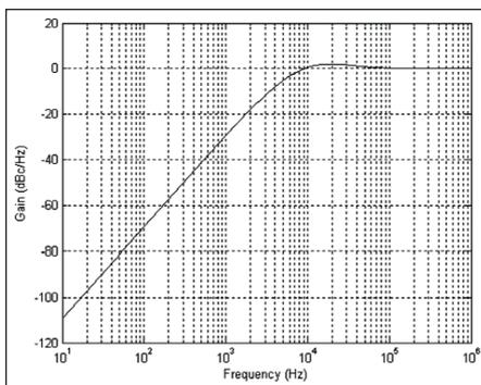
Figure 6 · Loop error response.
