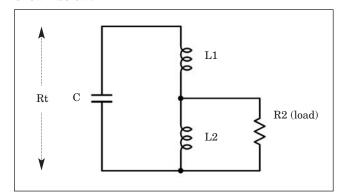
Since it is a complementary configuration, the analysis of the tapped inductor circuit is similar to that for the tapped capacitor circuit. It should be noted that a tapped inductor is really an autotransformer and as such has the properties of impedance transformation.
