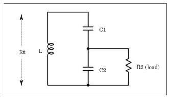
Here, R2 is the load across the tap. What is required is to find the values of L, C1, C2 when given R2, Rt,  $f_0$  and B.  $f_0$  is the resonant frequency, R2 is the load, Rt is the tank or terminal impedance and B is the bandwidth.
