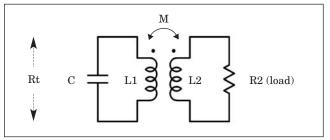
Experienced engineers may recognize this as "link coupling," which was commonly used in years past, and has been rediscovered for some integrated circuit applications.
