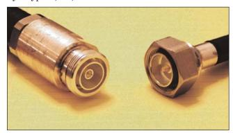
The name comes from the sizes of the inner conductor (7 mm) and outer conductor (16 mm). The connector is weather sealed, impedance-matched, and can be mated and unmated with those adjustable wrenches that are present in every technician's toolbox!
