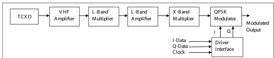
Figure 1 • Block diagram of the X-band data
