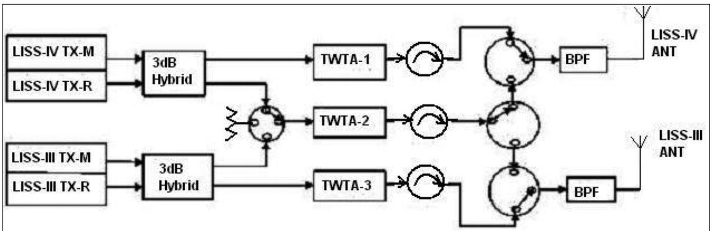
Figure 2 • Block diagram of the X-band data transmitting system.
