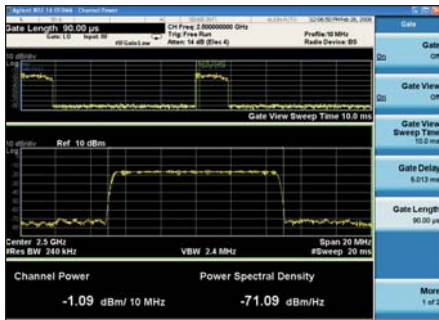
Figure 5 · The channel-power measurement above shows gating over the preamble only. This measurement is commonly referred to as the received signal strength indicator (RSSI) in WiMAX.
