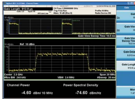
Figure 4 · The channel-power measurement above is gated over a WiMAX downlink burst consisting of one preamble and eight symbols.
