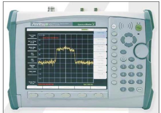
Handheld portable spectrum analyzers with high performance, like this Anritsu MS2721A, are among the recent developments by instrument manufacturers.
