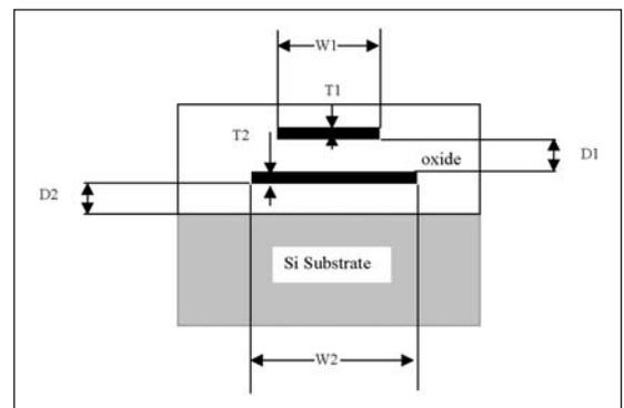
Figure 2 · Microstrip—substrate structure under study.  $T1$  = thickness of microstrip line and  $T2$  = thickness of ground return (bottom plate).  $D1$  is oxide spacing (height of microstrip substrate).  $D2$  is oxide spacing to the silicon substrate.  $W1$  is the width of the microstrip line and  $W2$  is width of ground return or bottom plate.
