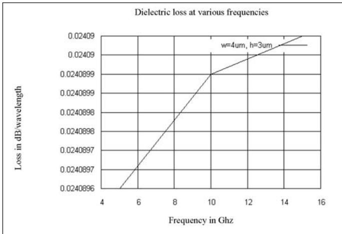
Figure 10 · Dielectric loss with varying frequencies for a 4 μm wide microstrip on a 3 μm thick oxide substrate.
