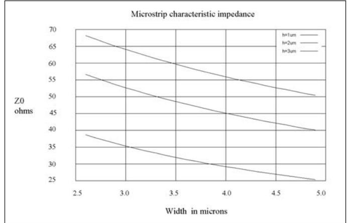
Figure 4 . Characteristic Impedance for varying width at 1 μm, 2 μm and 3 μm oxide thickness. Top curve is for h = 3 μm, middle curve is for h = 2 μm, bottom curve is for h = 1 μm.
