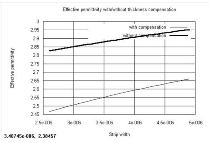
Figure 7 · Effective permittivity as a function of microstrip width with and without strip thickness as a parameter.  $h = 3.0 \mu\text{m}$ , thickness  $t = 2.8 \mu\text{m}$ .
