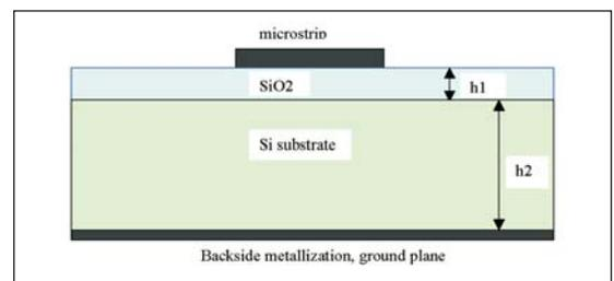
Figure 1 · Microstrip line on a silicon substrate with backside metallization and a layer of silicon dioxide.
