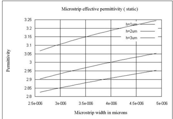
Figure 6 · Effective permittivity (static) variation with strip width ( $\epsilon_r = 3.9$ ). Top curve is for  $h = 1 \mu\text{m}$ , middle curve is for  $h = 2 \mu\text{m}$  and bottom curve is for  $h = 3 \mu\text{m}$  ( $h$  is the substrate thickness).
